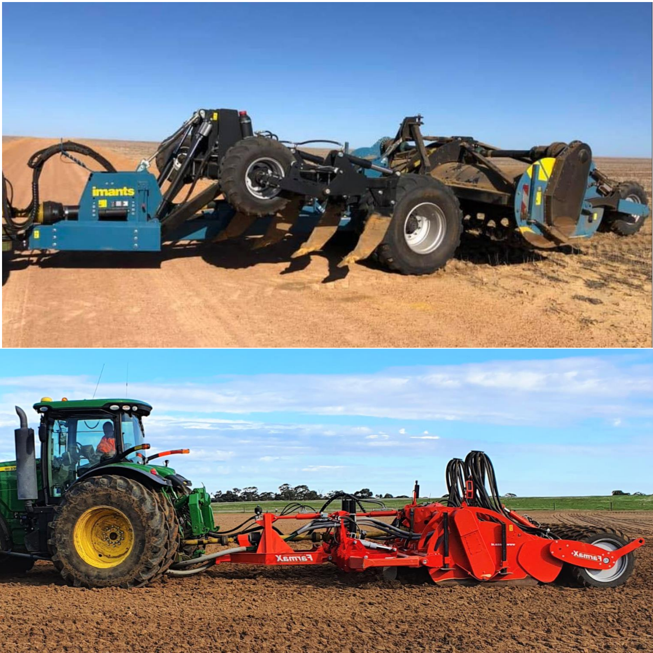
Photo 3: Combining deep ripping with spading in one-pass is now commercially available and allows complementary remedies to be applied towards multiple constraints within a deeper profile ; Images courtesy of Imants Spading Western Australia (top) and Farmax Spader - Groocock Soil Improvement (bottom)
